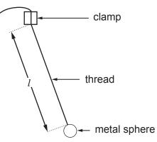
Using a metre ruler she measured the length, l, shown in the diagram. She then recorded the time for 10 small amplitude oscillations, repeated the timing and calculated values for the mean periodic time, T, and its uncertainty. She repeated the procedure for another five values of l. She plotted her values of  $T^2$  against l on the following grid.
