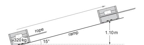
(a) Show that the mean *power* used to pull the piano up the ramp is approximately 120 W. [3]
